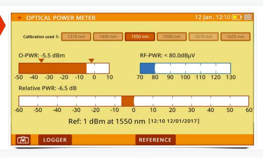
In this mode optical power measurement is shown together with the rest of the RF measurements. RFoG (RF-over-Glass) is used by CATV operators because it allows them to benefit from the advantages of fibre optics to compete with FTTH service providers.
